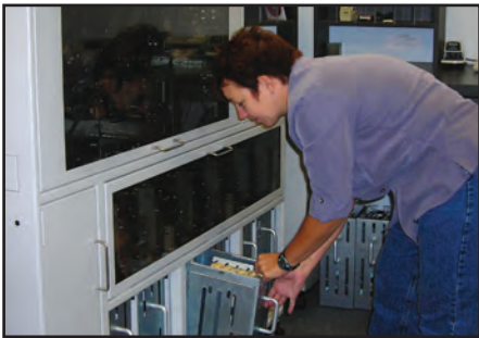
Peggy Johnson extracts configurable, 2000-note-capacity sorting cassette.
